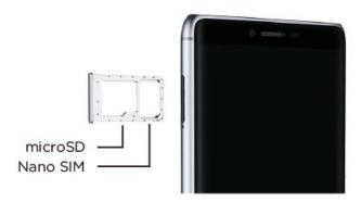
2. Gently pull out the SIM card tray. Place the Nano SIM card in card slot 1. If you have a microSD card (sold separately) place it in card slot 2.
