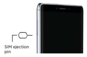
1. Insert the SIM ejection pin into the hole to open the SIM card tray.
