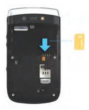
Slide the SIM card into the slot.
