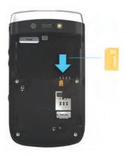
Slide the SIM card into the slot.
