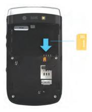
Slide the SIM card into the slot.
