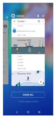
Touch one thumbnail and slide it up to close the application, slide it right/left to switch between the applications.
