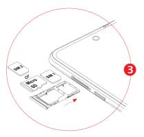
You must insert your SIM card to make phone calls. You do not need to power off your phone before inserting or removing the SIM card as this phone supports hot swap.
