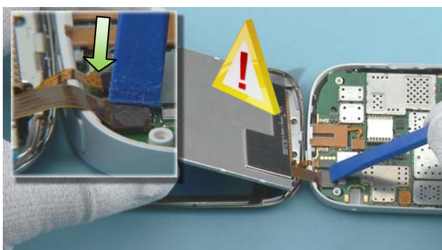
32) Hold the DISPLAY as shown and connect the connector with the SS-93. Be careful not to damage the connector, the flex or any nearby components!
