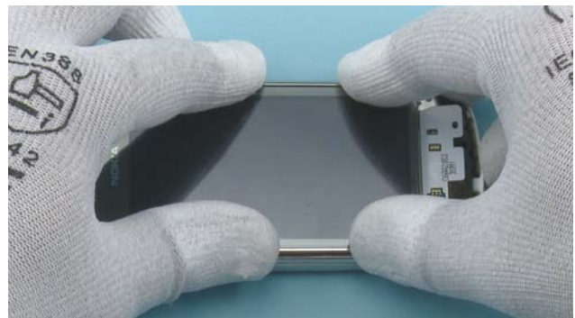
53) Place the A-COVER as shown and make sure that the A-COVER flex does not go between the edges of the A-COVER and the B-COVER.
