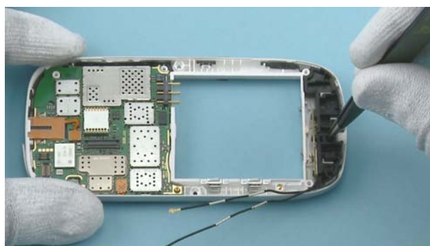
21) Place the MAIN ANTENNA with the tweezers.
