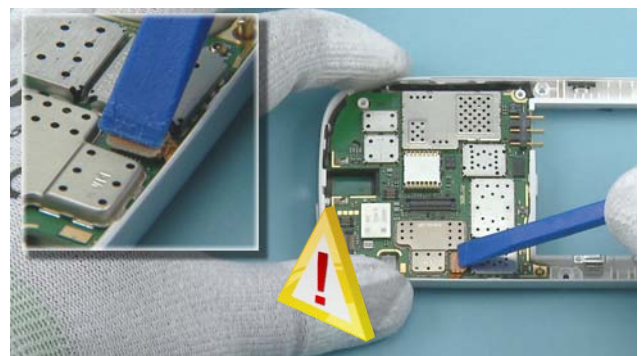
17) Connect the SIM CARD READER connector with the SS-93. Be careful not to damage the connector or components nearby!
