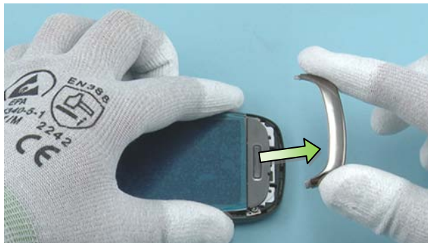
8) Remove the A-COVER CHIN by pulling it into direction shown.
