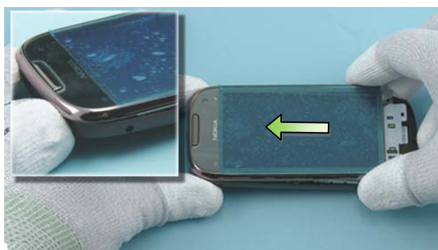
12) Release the A-COVER by sliding it very gently to the direction shown.
