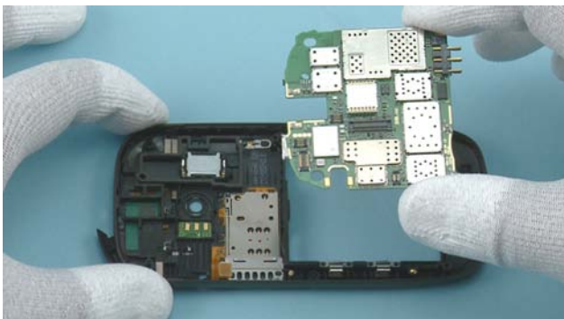
47) Remove the ENGINE BOARD.
