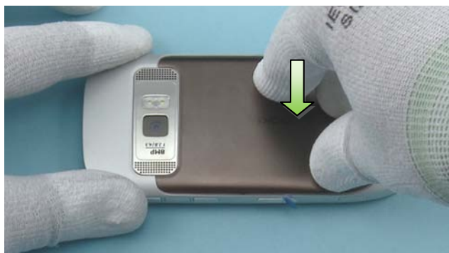
62) Then set down the bottom end and press it gently to lock it.
