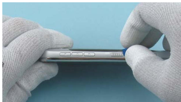
63) Finally, remove the LOCK KEY protective film.
