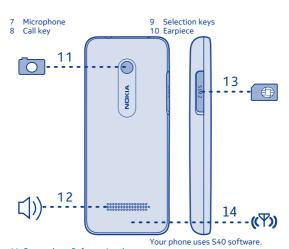
11 Camera lens. Before using the camera, remove the protective tape from the lens.
