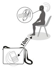
With Bluetooth wireless technology, you can connect your device, using radio waves, to a compatible Bluetooth device within 10 metres (32 feet).
